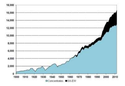
World copper mine production, 1900-2012 (in thousand metric tonnes)
